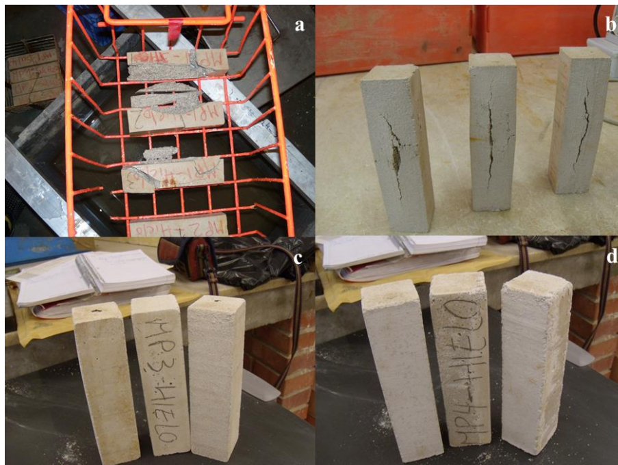
Figure 8: Mortars after being subjected to freezing-thawing cycles: a) control mortars after just 4 F-T cycles, b) 3% NS specimens after 6 F-T cycles; c) 10% NS samples after 6 F-T cycles, d) 20% NS mortars after 6 F-T cycles.
