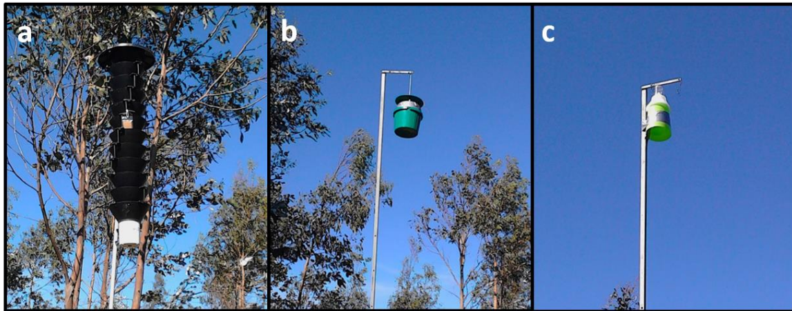
Figure 5. Traps used in the first field bioassay to trap Gonipterus platensis : (a) Lindgren multiple funnel trap, (b) unitrap and (c) boll weevil trap (photos taken by Luís Mota – RAIZ).
