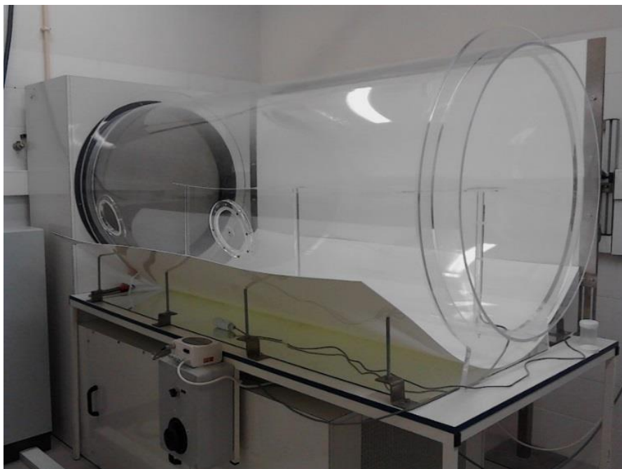
Figure 3. Wind tunnel used in the behavioural bioassays (photo taken by the author).
