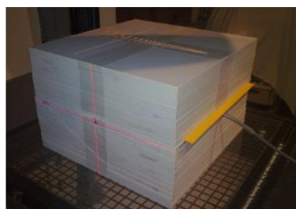
Figure 33 - Solid water phantom for verification with ionization chamber [25]
