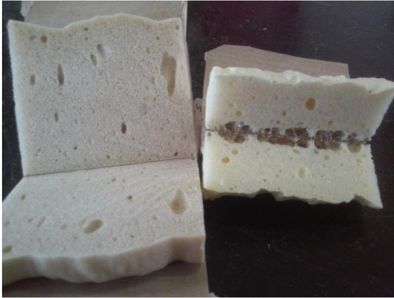
Figure 23 - Foams with base holes score 5 (left) and score -3 (right).
