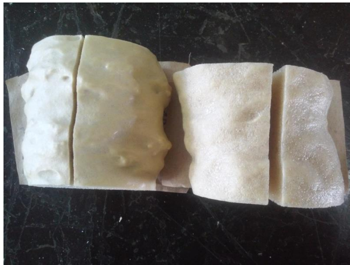
Figure 22 - Foams with glass bubbles score 5 (left) and score 3 (right).
