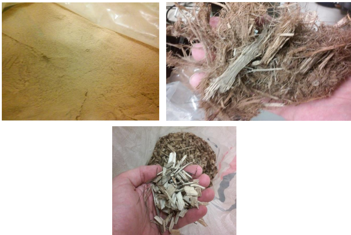
Figure 28 - Cork powder (top left), blue gum bark (top right) and poplar wood chips (bottom).
