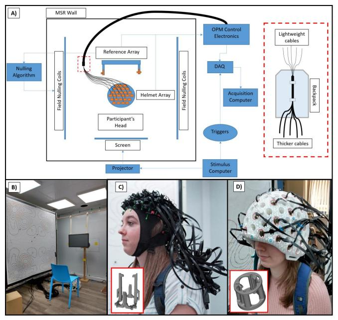
**Figure 1:– The OPM-MEG system.** A) Schematic diagram of the whole system. B) Magnetically shielded room. C) Flexible (EEG style) cap. D) Rigid additively manufactured helmet. Both helmets contain push-fit clips to house the 2<sup>nd</sup> generation QuSpin OPMs (shown inset in C) and D)).
