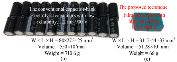
Fig. 18. Test set-up of (a) overall converter, (b) the capacitor bank for the dc capacitor storage technique, and (c) the film capacitor for the proposed technique.
