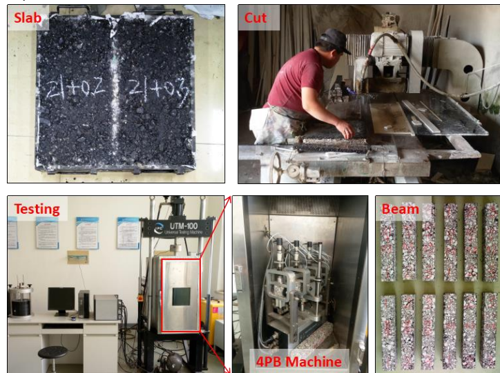
Figure 2. Sample preparation for 4PB fatigue test
