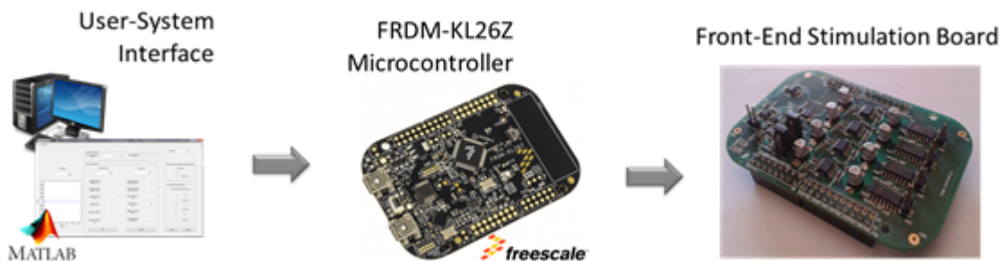
FIGURE 6.1: Overall Operation of the Embedded Platform for Neural Electrical Stimulation.
