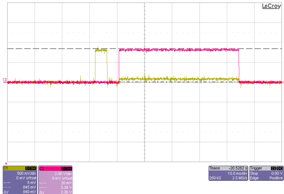
FIGURE 6.2: Measured wave for rectangular shaped stimulation.
