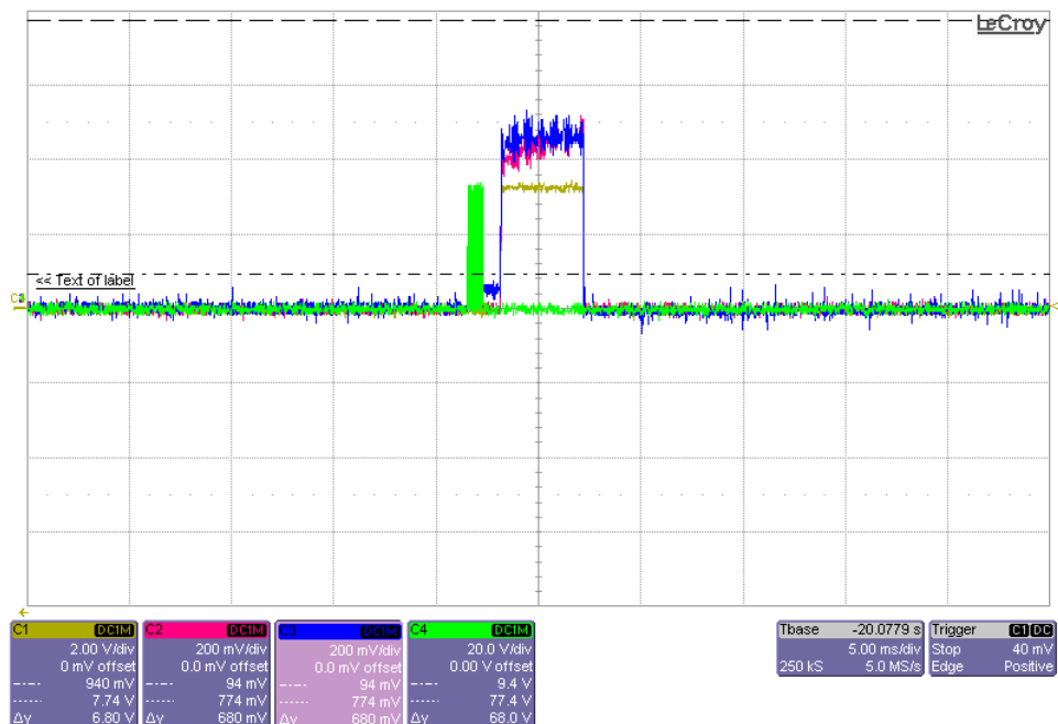
FIGURE 6.16: Charge-balancing results for Bursting Strategies based stimulation.
