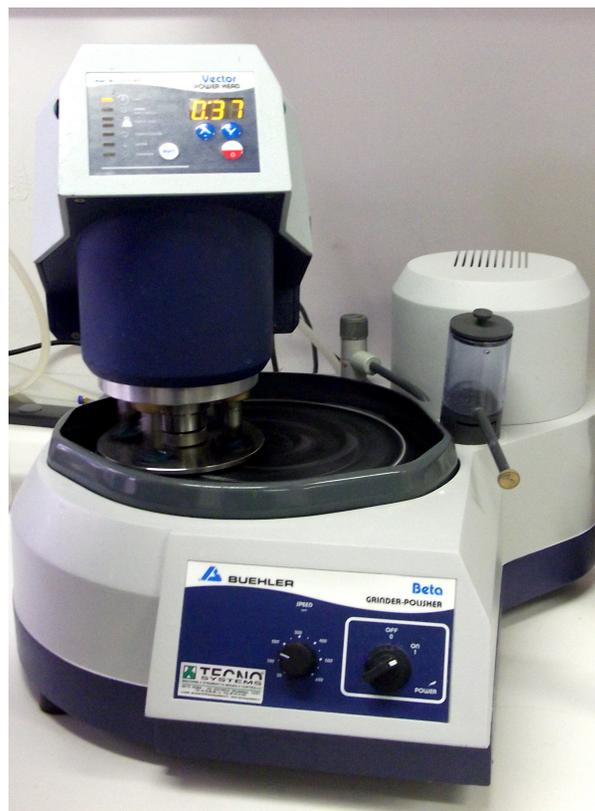
Figura 2.6: Moledor-pulidor vector/beta marca Buehler.
