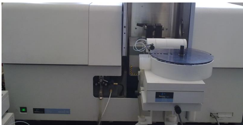
Figure 4 - Atomic Absorption Spectrometer, PerkinElmer Instruments AAnalyst 700.
