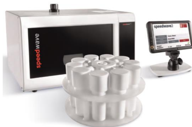
Figure 3 - Berghof Microwave Digestion System Speedwave Two (adapted from Berghof, 2014b).
