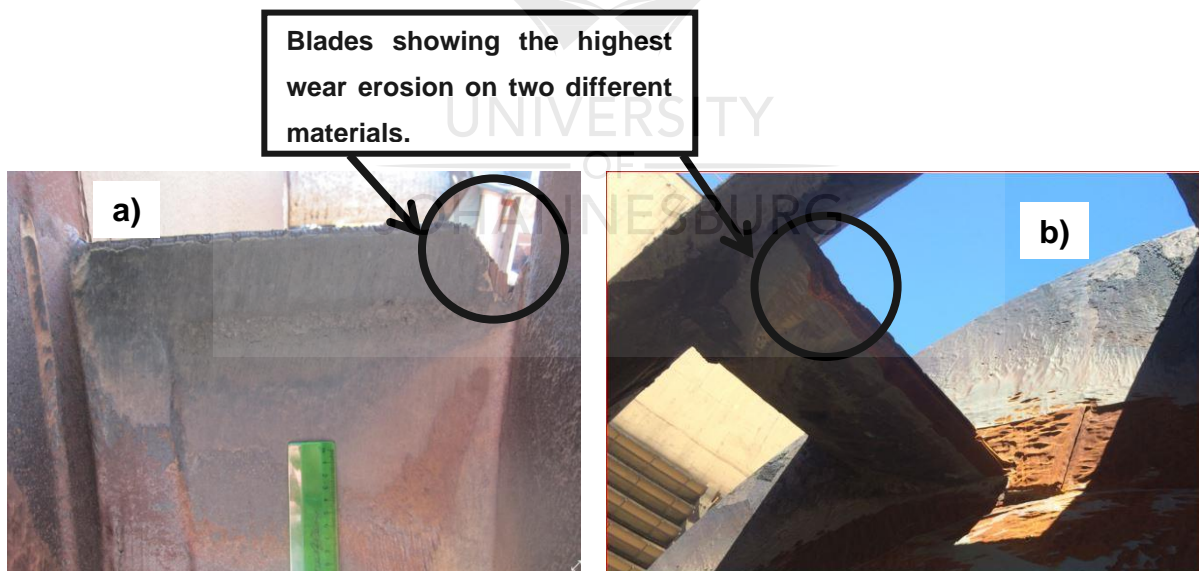
Figure 5 - 19: a) Blade made of Weldox 700 material. b) Blade made of S355JR material.
