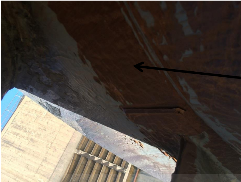
Figure C: Third picture showing wear on the backplate and hub plate.
