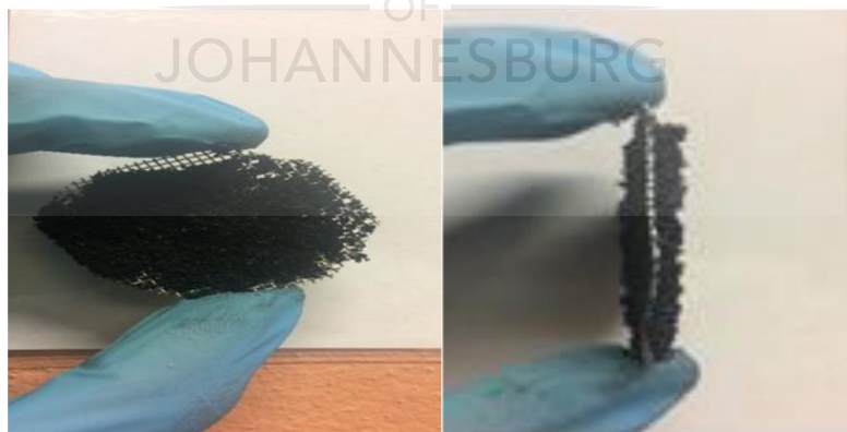
Fig. 1.1.3.1 – Activated carbon pressed to stainless steel mesh. (Schematic).
