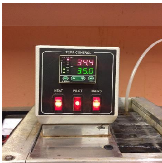
Fig. 3.3.3.1 – Temperature controller maintaining MFCs condition.
