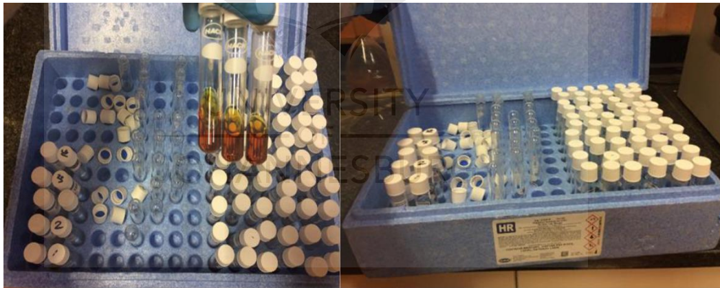
Fig. 3.3.2.1 – Before and after COD testing bottle for MFCs.
