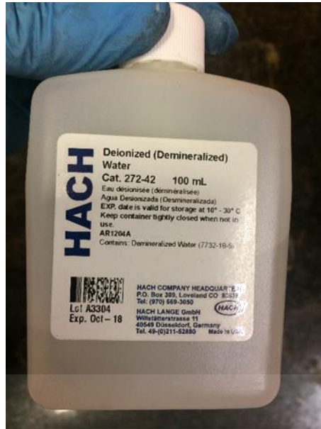
Fig. 2.5.1 – Deionized water for precipitation removal.
