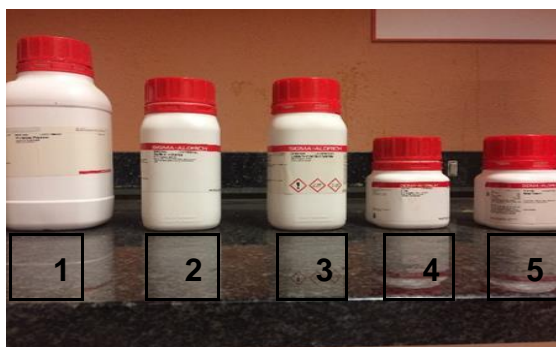
Fig. 3.2.1– Chemicals used for synthetic wastewater. 1) Peptone. 2) Sodium Chloride. 3) Calcium chloride dehydrate. 4) Urea. 5) Meat extract.
