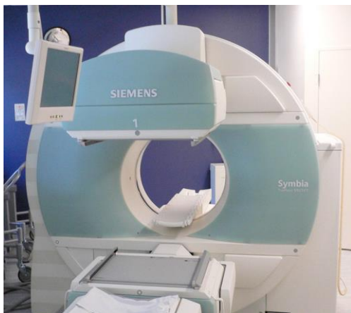
Figure 2. 1: Modern hybrid SPECT/CT scanner which incorporates multidetector CT (Hicks et al. 2007).
