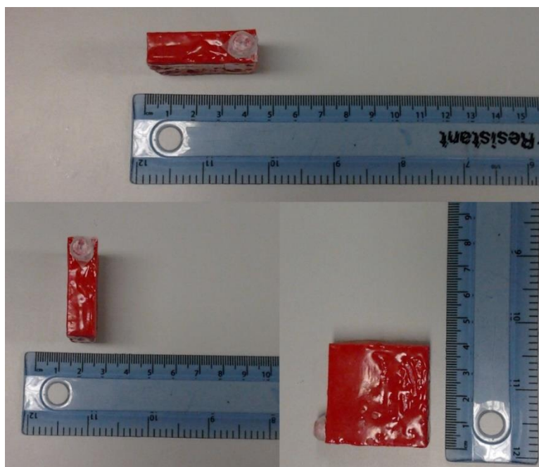
Fig 29 Three-way perspective of the separated small mpartment, after the epoxy resin had been applied.
