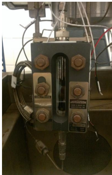
Figure 4.5– View of the high pressure cell of VLE apparatus #1
