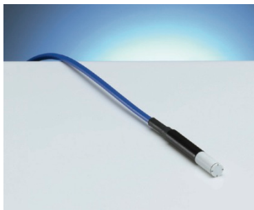
Figure 14: a) SCDD test unit of PTW. b) Schematic representations with the size of each part of the diamond detector. The red area (zoomed in) corresponds to the sensitive volume while the blue area to the capsule. The WET of the capsule is around 1.1 mm (adapted from [30, 32]).
