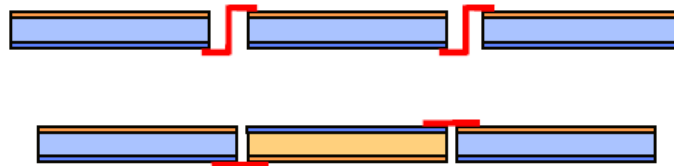
Figure 4 - Interconnection of p-type solar cells in a standard module (top) and of p- and n-type cells in a pn-module (bottom) [44]
