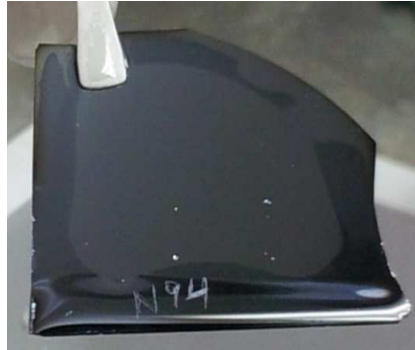
Figure 17 - Doped wafer after an HF dip. It is visible the presence of an hydrophobic behavior in the central region, while the borders are hydrophilic
