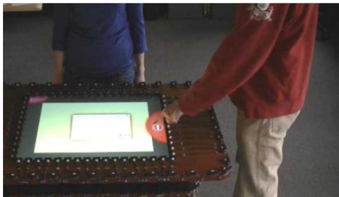
Figure 3.5: Medusa on "Do not disturb" mode. All logged out users are greeted with a "prohibited" glowing red orb [8]
