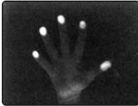
Figure 2.2: Infrared Light that escapes FTIR and is captured by the camera (image taken from [1])
