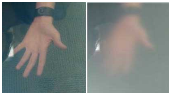
Figure 3.13: SecondLight switchable screen. Clear state (left) and diffuse state (right). (image taken from [17])
