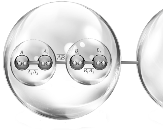
Figure 5.21: Illustration of renormalization in complex networks. Starting at connection \bar{A}\bar{B} between two clusters of agents, one scales down finding each cluster composed by two sets of agents, A_1 and A_2 on the left and B_1 and B_2 on the right connected again by \bar{A}_1\bar{A}_2 and \bar{B}_1\bar{B}_2 respectively. Each set of agents of this new scale can also be decomposed in two connected sets and so on downscale. For undirected networks, the number of probable states grows with N_p^2 , with N_p being the renormalized number of agents.
