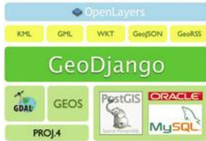
Figure 17 : GeoDjango Structure, including basic libraries, available databases, implemented standards and displaying format (Source:(Springmeyer, 2009)).
