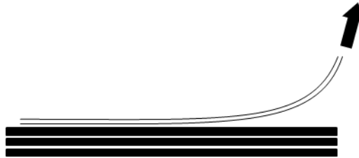
Figure 5 Sketch of a single fibre peel-off sample: a single fibre is glued on the top side of a UD composite material
