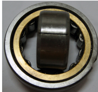
Fig. 9. The machined faulty bearing
