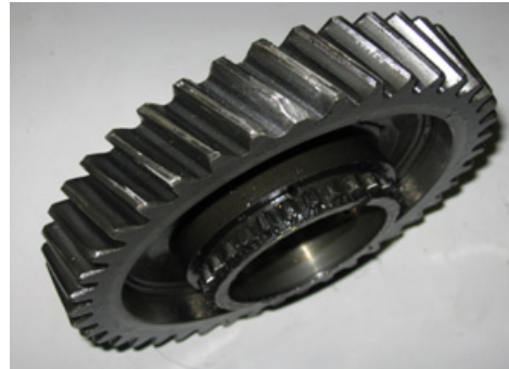
Fig. 18. The machined faulty gear
