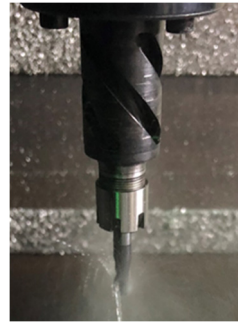
Fig. 13. Atomization on edge of cutter
