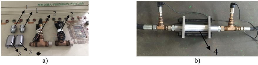
Fig. 4. Experimental devices of SEC and DTETC: 1 – union joints, 2 – pressure sensors, 3 – inserted tubes, 4 – expansion chamber cavity
