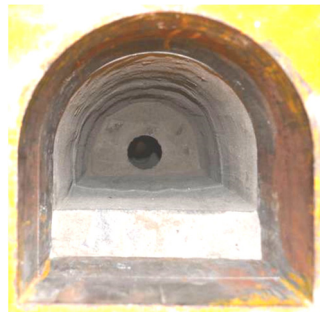
Fig. 6. Final excavated model tunnel
