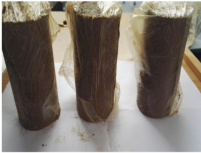
Fig. 6. Specimen in creep test
