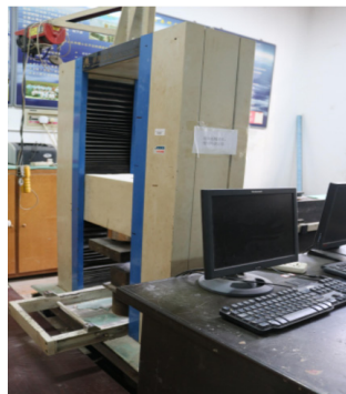
Fig. 2. RYL-600 rock shear rheometer test machine
