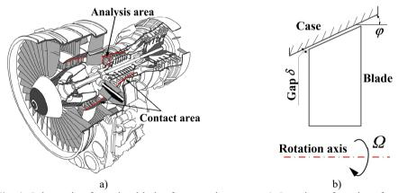
**Fig. 1.** Schematic of rotating blades force environment: a) Cut-view of an aircraft engine with sensitive contact areas [13] (https://doi.org/10.1115/1.4006446; Copyright © 2012 by American Society of Mechanical Engineers); b) Schematic of blade-casing
