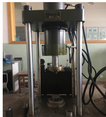
Fig. 2. Cold press molding equipment
