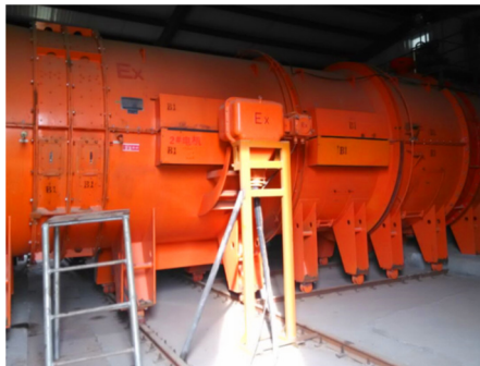
Fig. 1. The counter-rotating fan for testing
