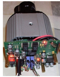
b) Picture of the camera and its control electronics
