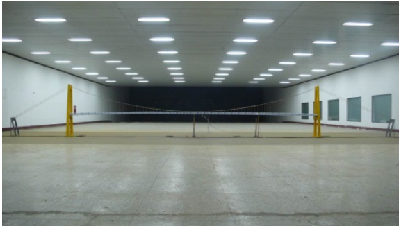
Fig. 9. Full aeroelastic model in wind tunnel
