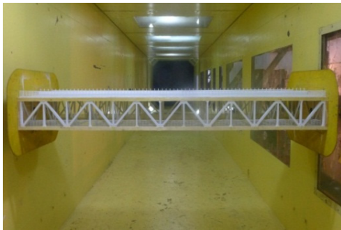
Fig. 3. Elastically-mounted sectional model
