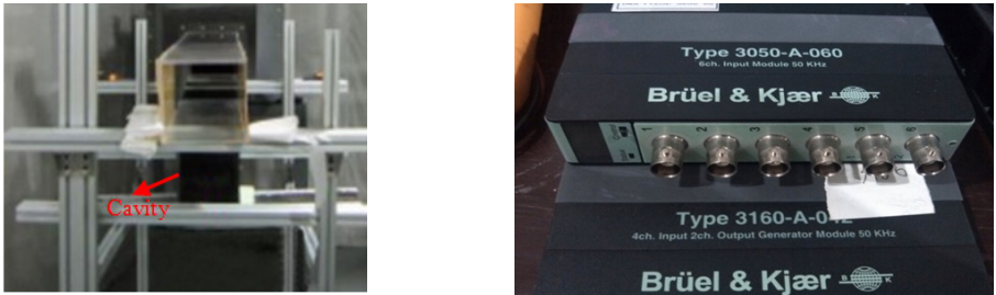
Fig. 9. Pressure pulsation test in the square cavity
