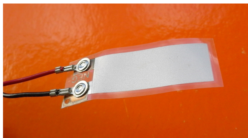
Fig. 3. Meas LDT1-028k transducer made of PVDF and silver
