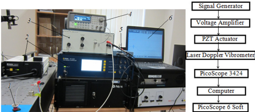
Fig. 7. Experimental set up. Here: 1 – piezoelectric deflector, 2 – laser Doppler Vibrometer Polytec TM, 3 – high voltage amplifier, 4 – signal generator Agilent 33220A, 5 – PicoScope-3424, 6 – computer
