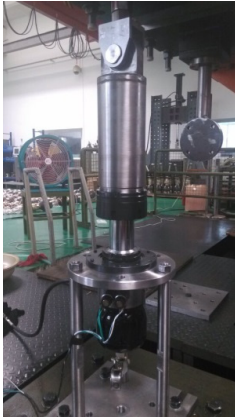
Fig. 2. Suspension bench test
