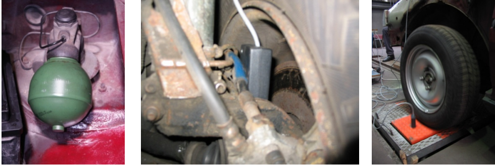
Fig. 5. Locations of vibration sensors during tests
