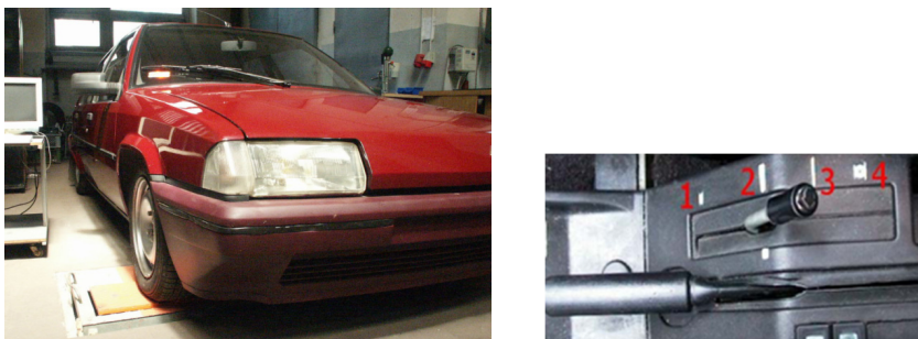
Fig. 4. Vibration test of Citroen BX 14 TGE and manual controller of vehicle clearance: 1 – low position, 2 – normal position, 3 – hard position, 4 – service position
