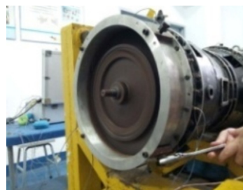
Fig. 2. Thick turbine casing single-point rubbing experiment
