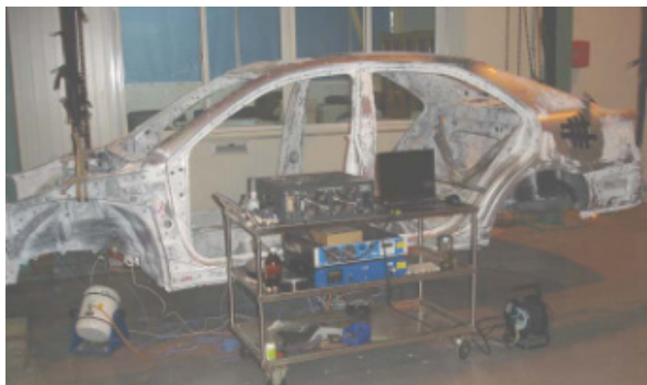
Fig. 7. Diagram of testing the experimental modal
