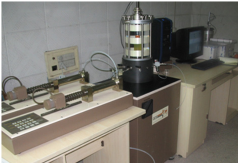
Fig. 1. GDS dynamic triaxial equipment
