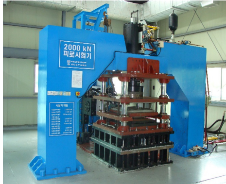
Fig. 7. 2,000 kN fatigue test machine
