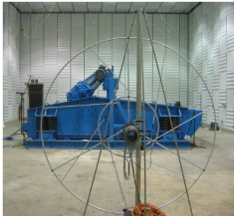
Fig. 9. Diagram of noise measurement for the vibration screen
