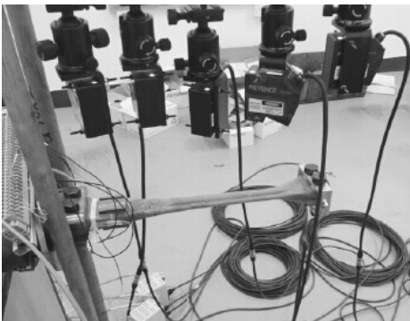
Fig. 1. Diagram of loading experiment in flapping vibration direction
