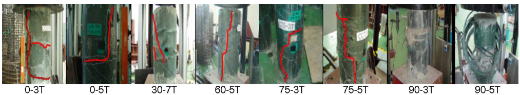
Fig. 5. Failure direction of uni-axial tests
