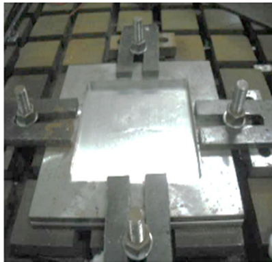
Fig. 9. Four-side fixation method in experiment
