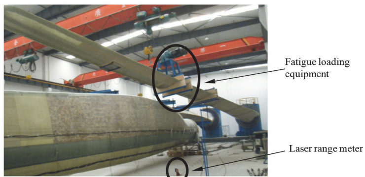
Fig. 3. On-site wind turbine blade fatigue loading test
