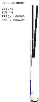
Fig. 7. The fourth mode shape
