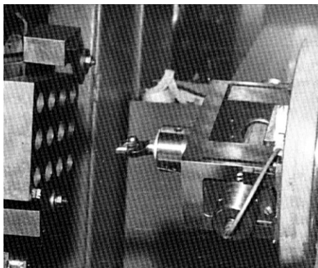
Fig. 4. The experimental CMA device for the stabilization of the oscillations of a boring bar in the process of aperture processing
