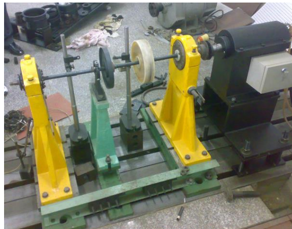
Fig. 1. The rotor test rig with oil-block inside the drum
