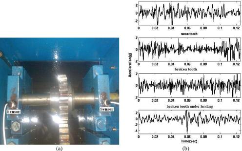
Fig. 4. (a) Experimental setup with the sensors, (b) time domain plot of signals
