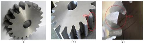
Fig. 3. (a) View of normal gear, (b) view of wear tooth, (c) view of broken tooth
