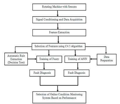
Fig. 1. The frame work of intelligent fault diagnosis system
